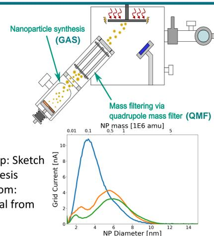
Figure 2: Top: Sketch of NP synthesis setup. Bottom: Typical signal from the QMF.
