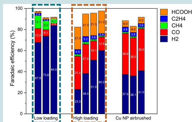
Figure 5: Faradaic efficiency of the catalyst over time for 3 different electrode designs. Changes over time demonstrate lack of catalyst stability in GAS-catalyst. The first catalyst corresponds to the 8nm, 300V bias deposition (Figure 4) and the second one to the cross-section (Figure 3)
