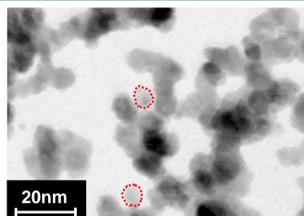
Figure 1: TEM micrograph of Cu NPs that were size-filtered at 8nm (provided by Michael Burtscher).
