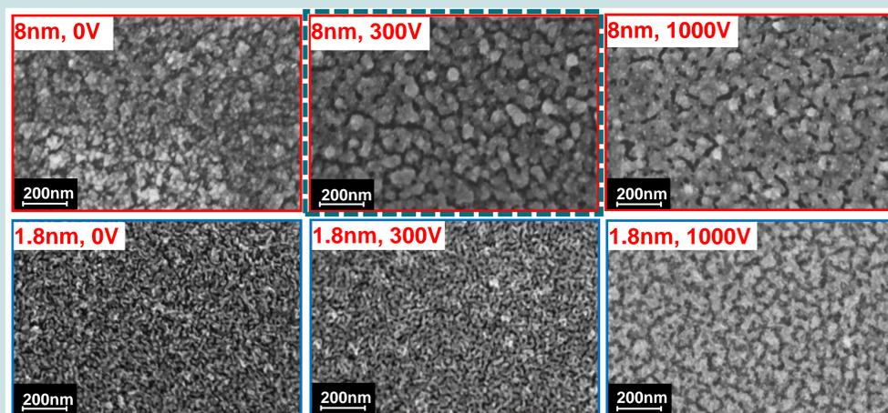
Figure 4: Left: QMF diameter profile (a), signal for 4nm filtered particles over time with bias (b) and derived mass flux of 1.8nm and 8nm filtered particles. Right: Top-view SEM micrographs of the depositions corresponding to the mass-flux graphs shown in Figure 3 (c)
